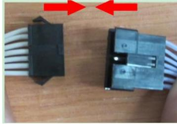
**FIG-17** Connecting control panel connectors
