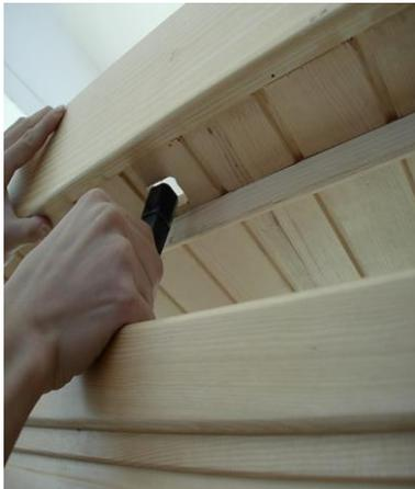
**FIG-13** Slip cords/wires through corresponding holes
